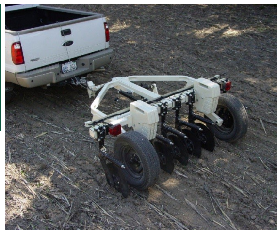
Figure 11. Veris electrical conductivity sensor. (Photo courtesy of Veris Technologies, Salina, Kans.)
