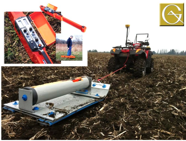
Figure 13. Electromagnetic sensors. (Photos courtesy of Geonics, Ltd, Mississauga, Ontario, Canada)
