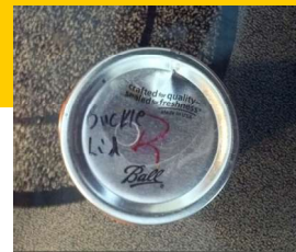
Buckled lid – ring screwed on too tight
