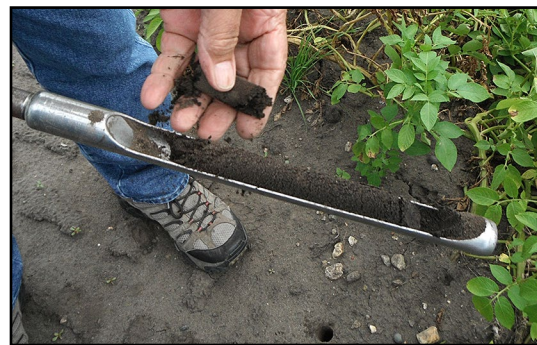
Testing soil moisture in the top 6 inches with a soil probe. (Tom Scherer, NDSU)
