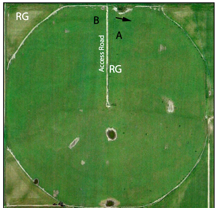
Figure 2. Ideally, each center pivot should have two rain gauges, one in the dryland corner and one along the access road about halfway to the pivot point. Soil moisture deficit should be measured near the starting point of the center pivot (A) and near the last part of the field to be irrigated (B).
