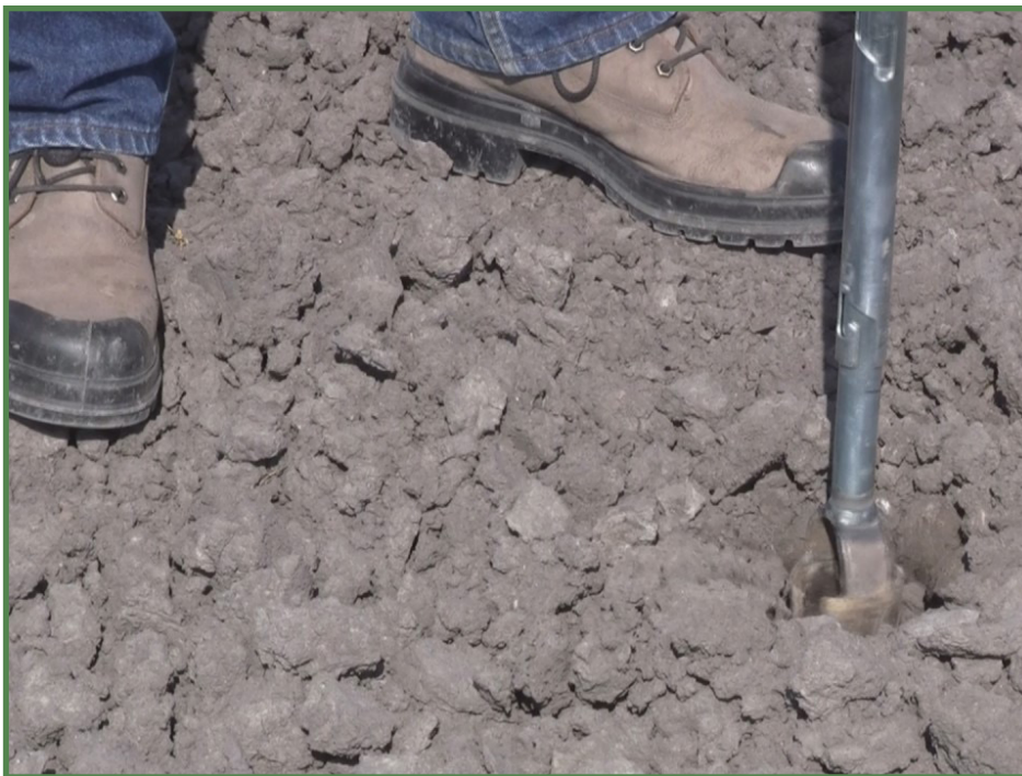
Figure 4. A soil core is being taken from a saline-sodic zone with a hand-held auger. (Naeem Kalwar, NDSU)
