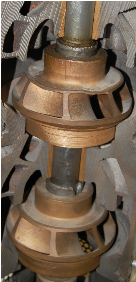
Figure 5. Cutaway view of two enclosed impellers within their pump bowls.
