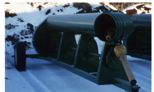
Figure 9a. A power-take-off (PTO) driven propeller pump used to move large volumes of water in low lift conditions.
