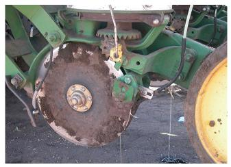
Photo 2. Planter set for in-furrow fertilizer placement. (Greg Endres, NDSU)
