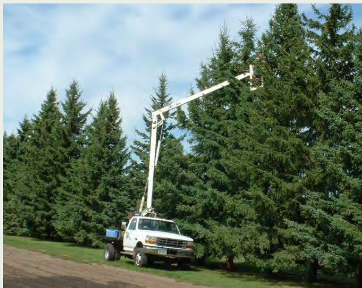
Fig 3 A boom truck is used to pick cones (photo courtesy of Jeff Smette)
