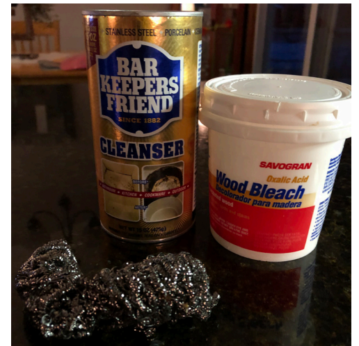
Fig. 2 The materials needed to remove or diminish the water stains included a stainless steel scrubber, Bar Keepers Friend cleanser and oxalic acid.
