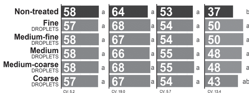
Figure 1: When the soybean canopy closure averaged less than 75% at fungicide application at the R2 growth stage, fine to medium-fine droplets optimized fungicide performance in the only study in which statistical separation of treatments was observed. Within-column means followed by different letters are significantly different ( P < 0.05 ).
