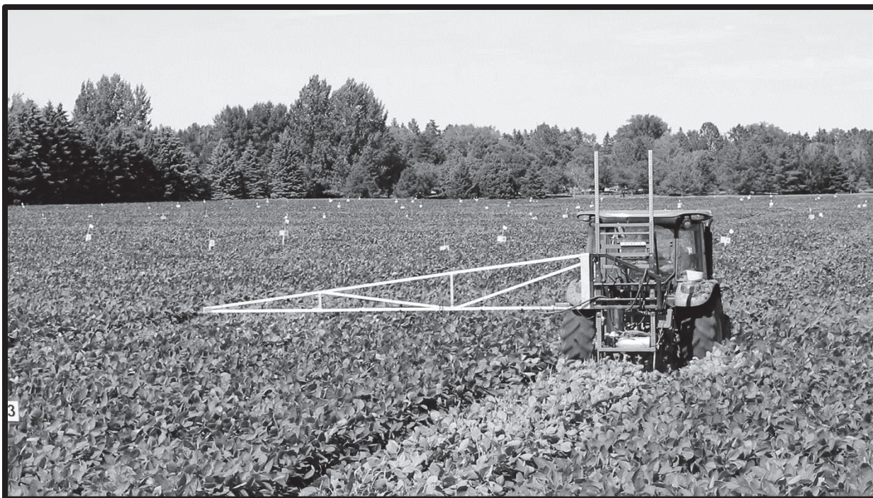
Making applications with the tractor-mounted sprayer to the droplet size studies in Carrington in 2019. Flags mark the start and end of the treatment plots. To prevent edge effects, alleys were not cut between plots until harvest.
