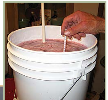
▲ Taking a specific gravity reading using a hydrometer
